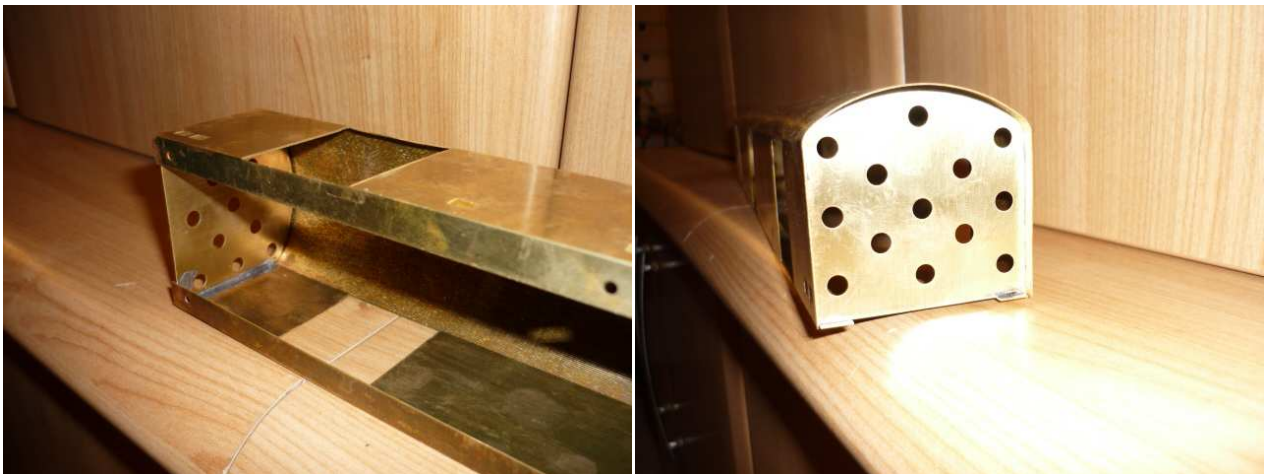
Ends Soldered in Place (Note you can see two of the holes which you need to solder the chassis retaining nut to inside the body)
