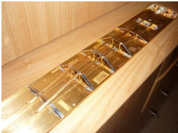
Cross Truss Fillets
